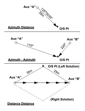
Distance Distance: Enter Distance and Delta Ht for 1st position from Aux Pt A; repeat for position B and choose the solution method (i.e. Left or Right)
